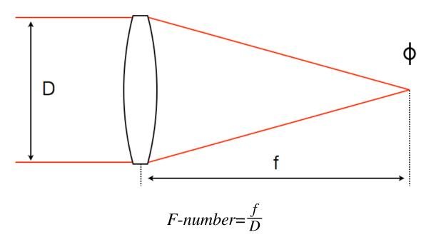
If the area of the aperture is doubled, the number of photons that can reach the sensor through the lens is also doubled. The F-number of a lens is the ratio of its focal length divided by the diameter of the aperture. Since the F-number is a ratio involving the diameter, and not the area, we lose the ability to nicely double or halve a number to calculate a stop.
