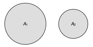
$A_1$  is twice the area of  $A_2$ , and we will assume that the diameter ( $d_1$ ) and focal length (f) of  $A_1$  is 1, so the F-number would be 1. Let us further assume that the focal length of the lenses are the same. To figure out the F-number of  $A_2$ , we need to determine how much smaller the diameter is compared to that of  $A_1$ . Let's do the math!
