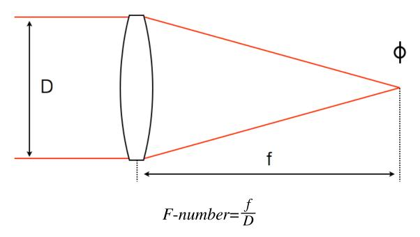
If the area of the aperture is doubled, the number of photons that can reach the sensor through the lens is also doubled. The F-number of a lens is the ratio of its focal length divided by the diameter of the aperture. Since the F-number is a ratio involving the diameter, and not the area, we lose the ability to nicely double or halve a number to calculate a stop.
